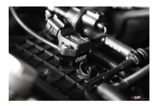
Lubricate the O-Ring on the O-TAP B body with engine oil and secure both sensor and the O-TAP B into the intake manifold with the supplied long screws.
